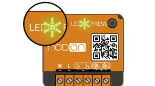
3a The LED of the relay switch will blink green twice, confirming the pairing of the two devices.
