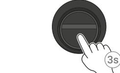
2 You have 30 seconds to pair your Floor Switch by pressing the button for 3 seconds.
