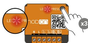
1 Launch the pairing by doing 3 consecutive presses on the relay switch button. The LED blinks red.
